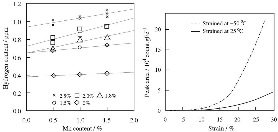
Figure 8: Left: effect of strain and manganese content on the amount of hydrogen absorbed in identical conditions. Right: effect of the temperature at which the material is strained, on the amount of hydrogen subsequently absorbed in identical conditions. After Nagumo *et al* [32]
