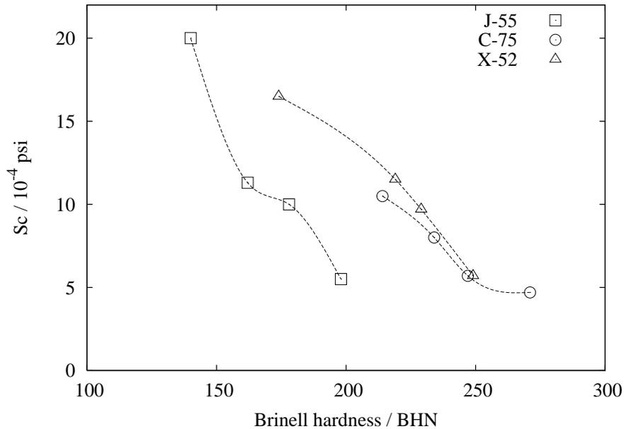
Figure 3: The effect of hardness increase (caused by cold working), on the SSC susceptibility of three API grade steels. Increases in hardness were obtained by cold rolling to 4, 8, 16 and 32% thickness reduction. After Treseder and Swanson [13].
