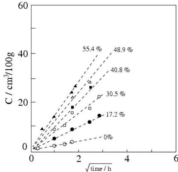
Figure 7: Hydrogen concentration as a function of exposure time to an aqueous  $\text{H}_2\text{SO}_4$  solution. After Hudson and Stragand [29]. Cold work increases the amount of hydrogen absorbed and the rate of absorption.
