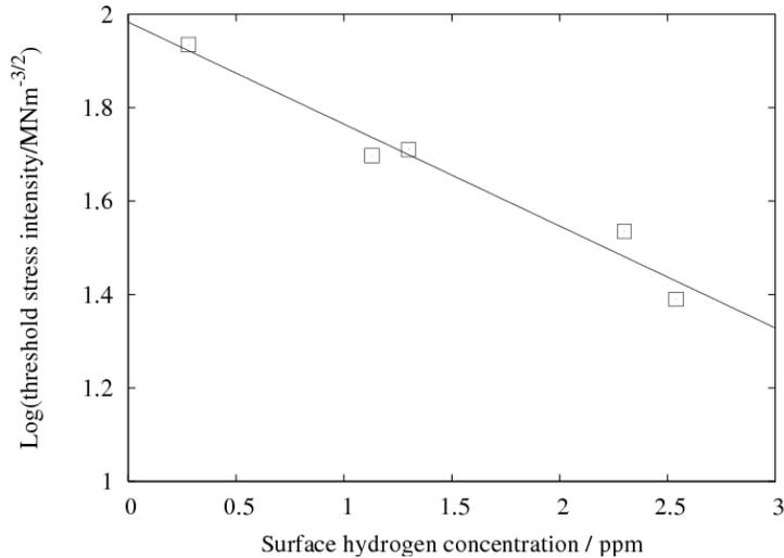
Figure 9: The influence of hydrogen content on the threshold stress intensity for steel BS4360 Gr50D, with a hardness of 405 HV ( $\pm 25$ ). After [33].
