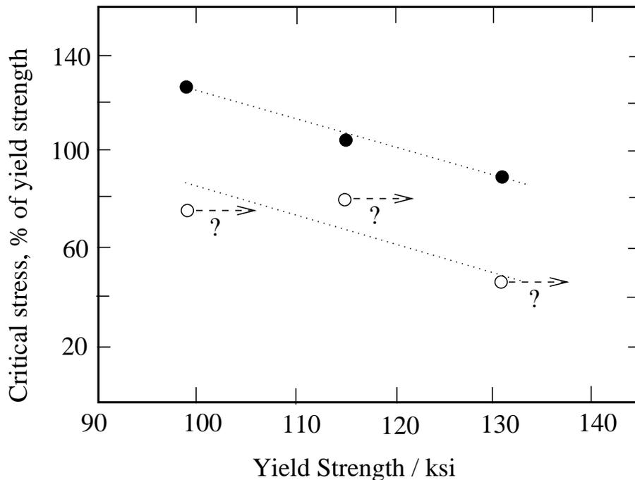
Figure 4: The effect of cold working on the critical stress for SSC in saturated  $H_2S$  solution. After Dvoracek [14]. Filled circles are for unstrained material, empty circles for cold-worked. As in Dvoracek's work, the data for cold-worked material are shown assuming the yield stress has not been affected. This is, however, unlikely to be correct, as illustrated by the question marks indicating a possibly higher yield stress value.
