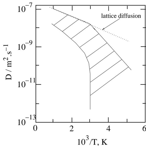
Figure 6: Range of diffusivity of hydrogen as a function of temperature, illustrating the role of reversible traps at low temperatures. After [28].
