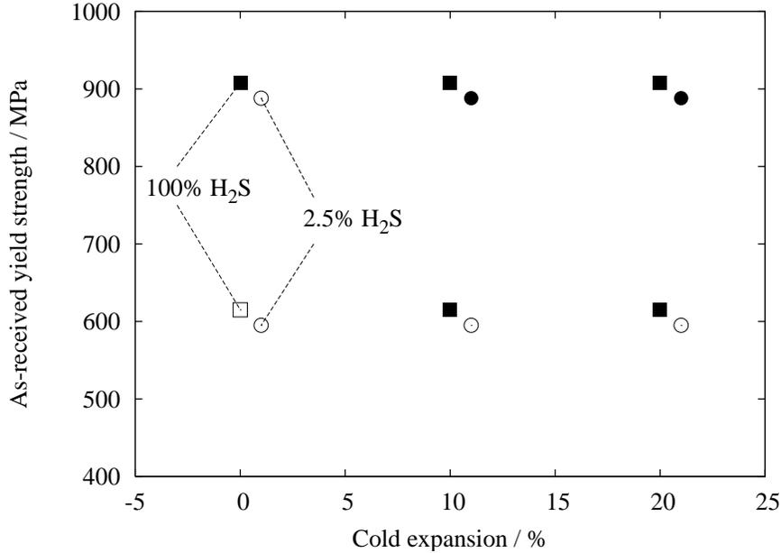
Figure 5: Outcome of SSC tests in 100% H<sub>2</sub>S (squares) and 2.5% H<sub>2</sub>S (circles) solutions, for L-80 and P-110 pipe materials, using data from [16]. Empty symbols indicate a pass, filled symbols a fail.
