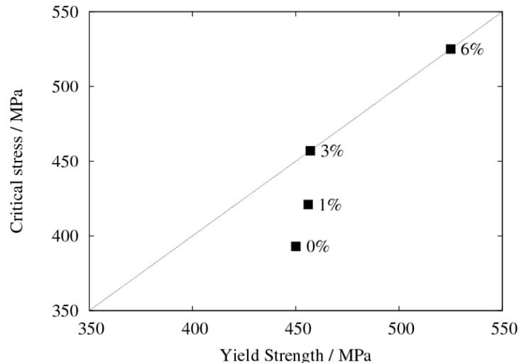
Figure 2: The critical stress for the SSC of a low strength steel as investigated by Asahi *et al* [10]. Cold work appears to result in an increase of the critical stress.
